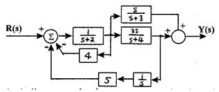
Use block diagram reduction to rearrange the above block diagram into the form shown below (i.e., H configuration) and find its transfer function,  $\frac{Y(s)}{R(s)}$ .
